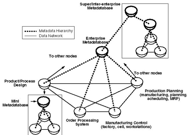
**Figure 5 : Enterprise Integrated Through Distributed Metadatabase System**
