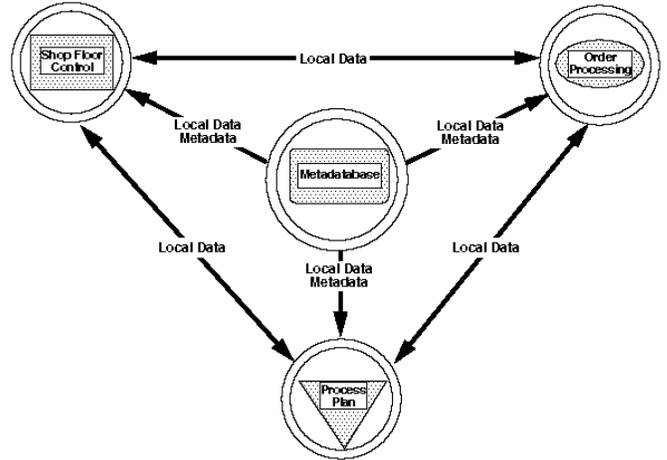
Figure 1 : The Concurrent Architecture Using a Metadata Database
